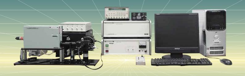
Data are aquired by the combination of a photomultiplier detector and a digital osciloscope in the single-wavelength monochromator system, and by the combination of a photodiode array detector and a high-speed AD converter in the multi-channel spectrophotometer system. In both systems, time resolution up to 10 nsec is available.
